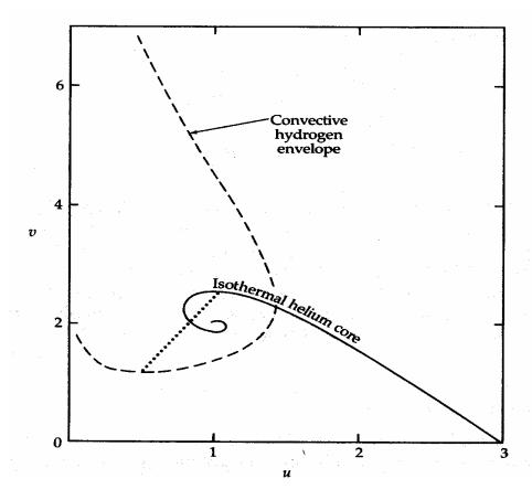
**Figure 2.3** represents a model star composed of two polytropes. The outer convective hydrogen envelope can be represented by a polytrope of index n = 1.5, while the helium core is isothermal. The discontinuous change in u and v resulting from the change in chemical composition can be seen as a jump from the isothermal core solution toward the origin and the appropriate M-solution for the envelope. Such a model can be expected to qualitatively represent the evolved phase of a red giant.
